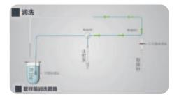
· Continuous sampling, dual sample sampling, automatic sample dilution and other functions Automatically rinse the pipeline and sampling pump before sampling to ensure the accuracy of sampling.
